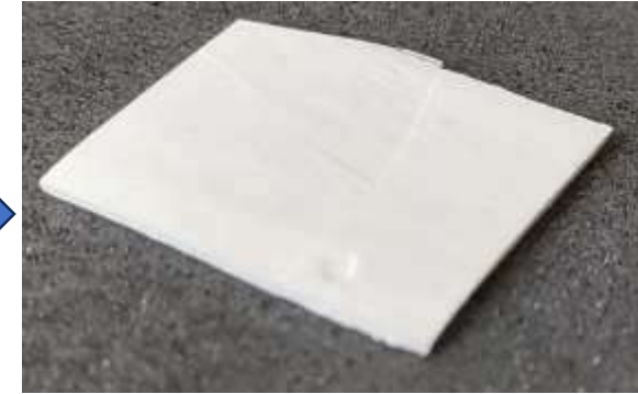
Figure 11. Thin Film Catalyst Coated Ceramic Plate
