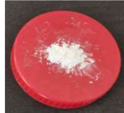
Figure 10. K-AS50 Al/Si Based Solid Catalyst Powder (< 8μ)
