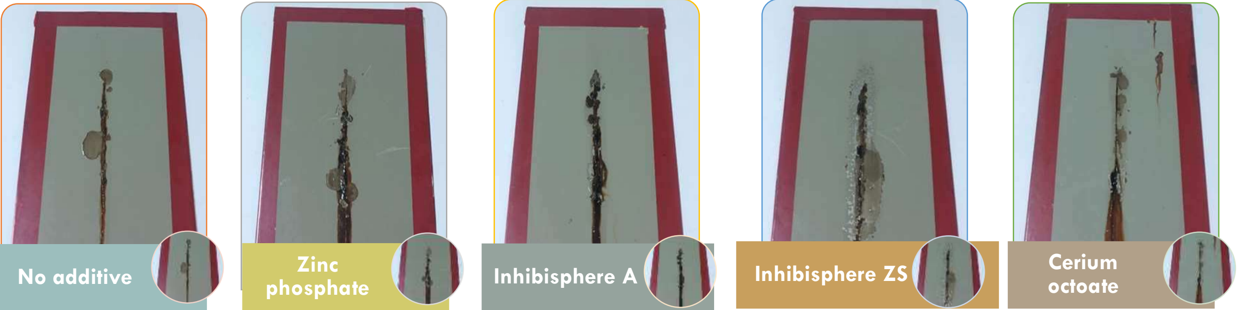
Figure 3: Panel's photographs after 500 hours corrosion test
