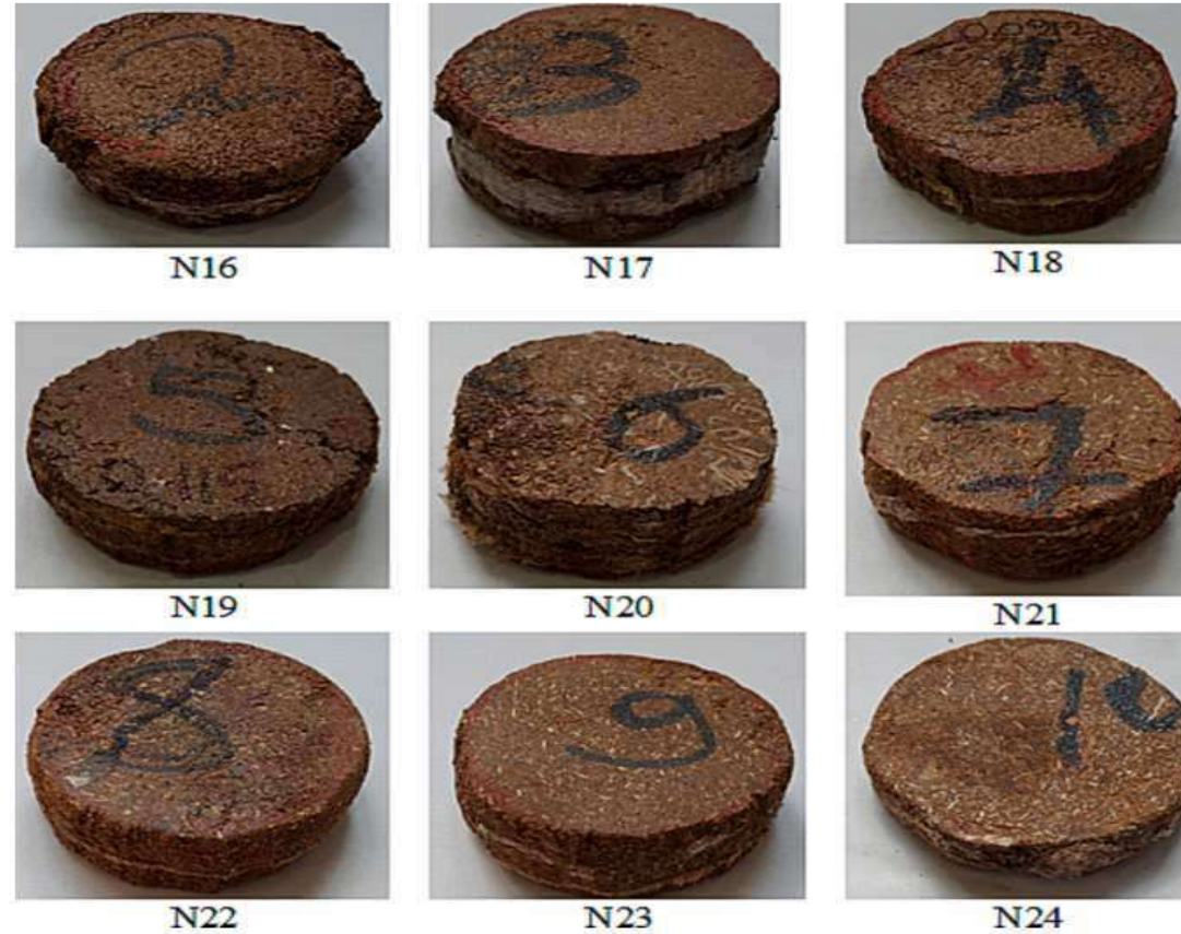
Fig. 10. Appearances of the some specimens as a result of the compression test (initial sample 6 cm diameter and thickness 2 cm).
