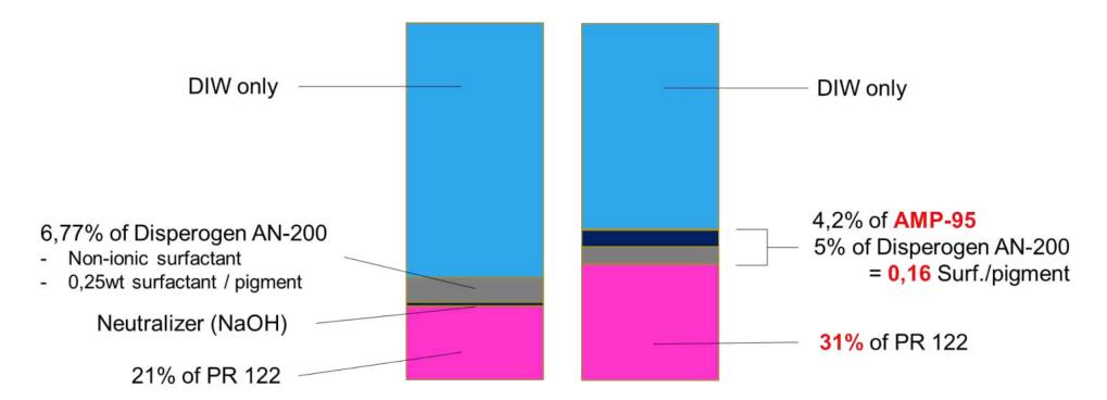
Formulation in water only 50% replacement of conventional dispersing agent with AMP Side-by-side comparison with the same viscosity => Optimization of the solid content
