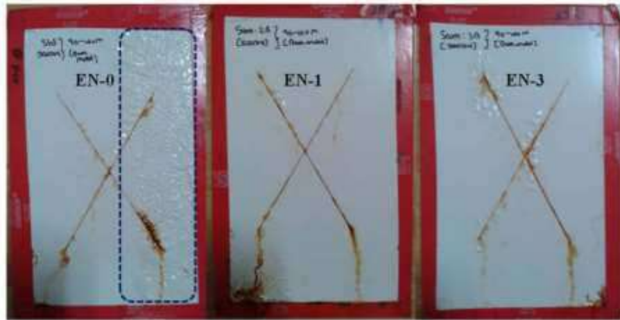
Coated panels after 500 h salt spray chamber [3]
